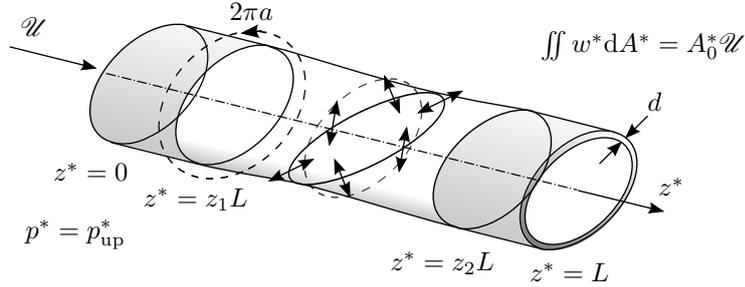
**Fig. 2** The set-up used in (31). An initially elliptical elastic-walled tube is clamped between two rigid tubes. Fluid flows from left to right, due to a volume flux condition at the downstream end.
